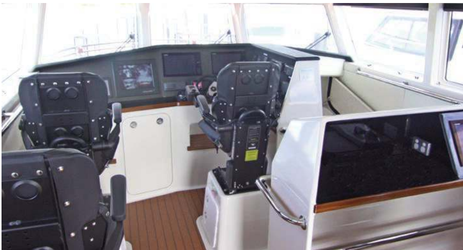
Above: The wheelhouse featuring Shockwave's shock-mitigating seats
