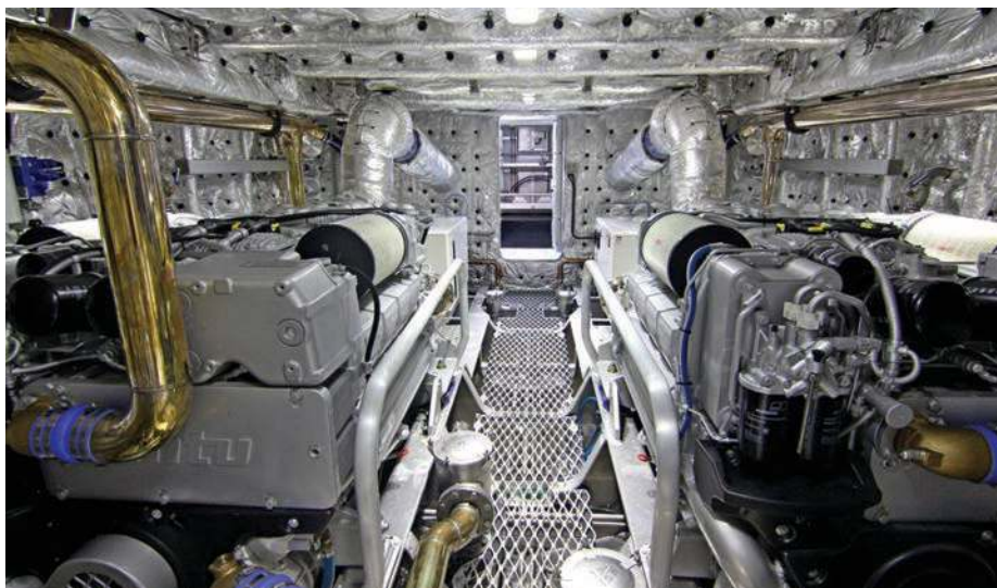
Below: The twin MTU 8V 2000 M72 engines powering the 19.2-metre 'AMG Winyama'
